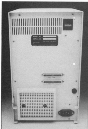
All connections to the BBC are made via ribbon cables — 2 sockets on the back and one on the side.
